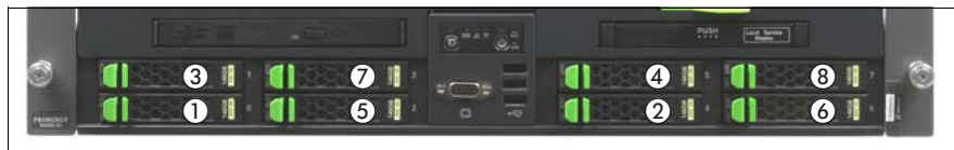
Figure 247: Mounting order for HDD/SSD bays
